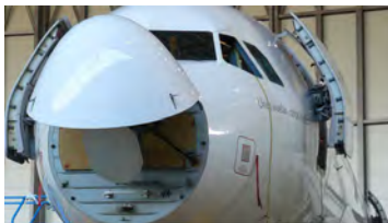
nose radome and radar antenna
