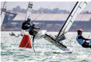
Nacra 17 boat flying : only the foils are immersed
