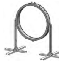
Custom-designed testing tooling for the uniform application of anti-corrosion treatments inside the cooling envelopes.
