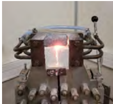
45S5 glass synthesis by melting
