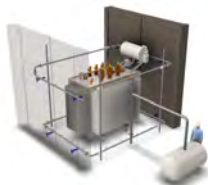
Initial extinguishing system, operating with pressurized water from the tank to the extinguishing lines around the transformer.
