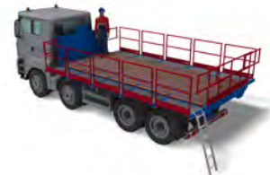
The device is unfolded from the dock for securing access.
